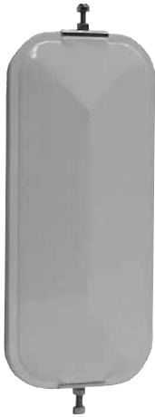
W-180 7" x 16" Steel Head (White) with 5/16" stud
