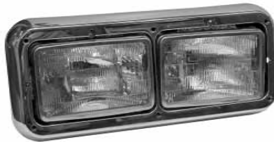
921-3310 - Dual Halogen Headlight System with chrome trim bezel and 2 foot wire lead. Universal in design with low beam on one side and high beam on other. Reverse headlamps for other side of truck. Overall Dim: 16" x 7". Fits in opening 5-3/8" x 14-3/4" x 3" deep.
