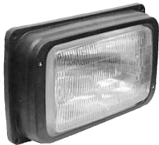
95-152 - Hella Headlight capsule with frame, uses B-9004 bulb. Overall Dim: 8-1/2"H x 13-7/8"W; Mounting Holes on 7-1/2" and 11-5/8" centers
